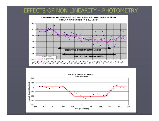
As an example of the effect of improved linearity on scientific measurements, consider a high precision photometry application such as exoplanet transits which require a precision of better than 10mmag for periods of several hours during changes in object altitude and sky conditions.
