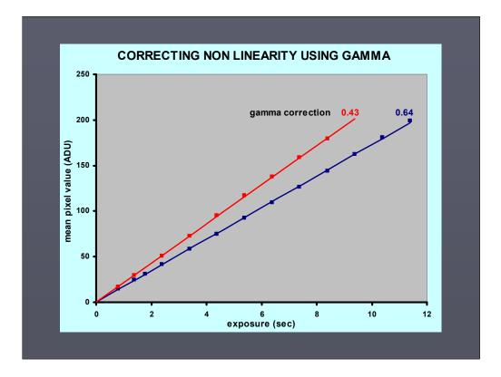
By applying an inverse gamma correction to the images (both dark and light) it proved possible to correct the response of the camera to produce a linear result at any given gamma setting.
