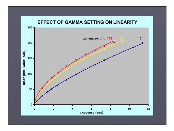
Linearity was measured by taking a series of exposures of different lengths with the light at constant brightness (light). The camera output at zero light levels (dark) was also recorded for each exposure time and subtracted from the corresponding light.
