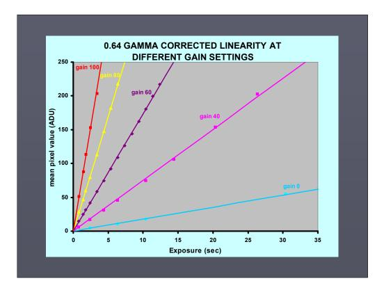
To test whether this result was true for all gain settings, a set of runs was made at 0 gamma and for a range of gains.
