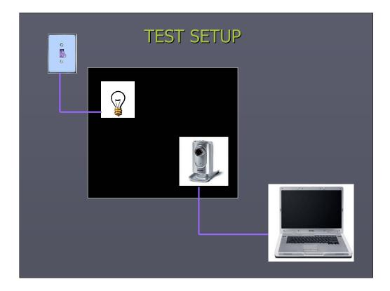
The test setup consisted of a light tight box containing the webcam and a very dim light source wit ha means of switching it on and off and varying the light output. (Long exposures of several seconds are used for the measurements)
