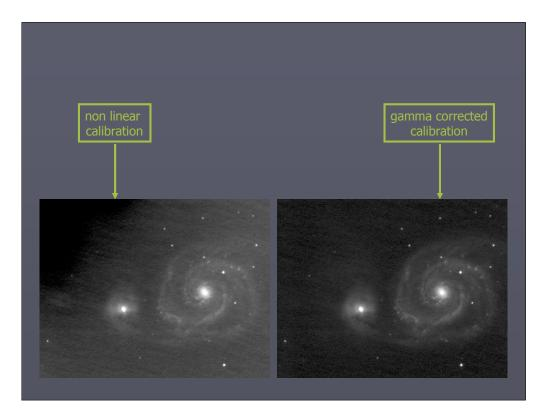
The background is noisy in both calibrated images due to a noisy flat (taken, using the T shirt technique, too late in the fading twilight) The beneficial effects of linearity correction on the amp glow and dust donuts are still clear however.
