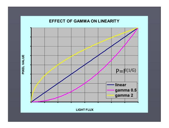
Unlike astro cameras which are normally designed to be as linear as possible, webcams have an adjustment specifically designed to make the camera non linear ie the gamma adjustment.
